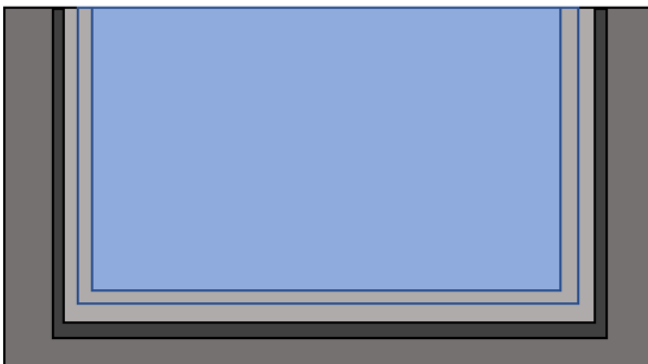
Figure: Pond walls with double inner layer of ceramic brick, 19mm bitumen lining, 300mm exterior concrete
